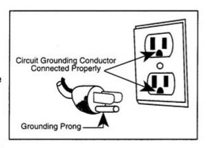
used in combination with a properly connected grounding-type outlet as shown in the figure.
